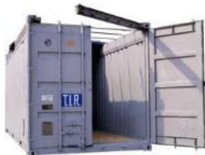
Figure 3.21 – 20-foot open top with tilt removed and rear header open
