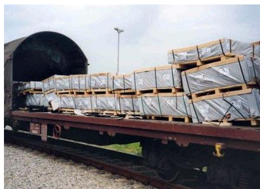
Figure 1.7 – Loose packages on rail wagon
