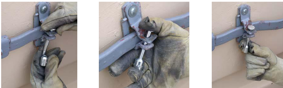
Figure 9.25 Fitting a bolt seal
