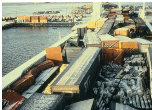
Figure 1.4 – Shifted cargo on a ro-ro deck
