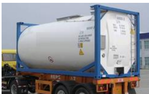
Figure 3.41 – 25,000 l collar tank
